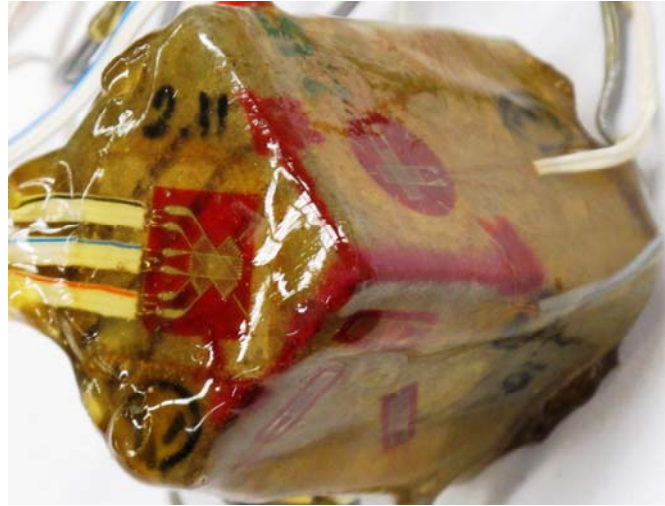
Figure 1: Specimen for jacketed compression test.
